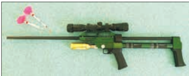
3.4 Carbon dioxide powered dart gun for remote delivery of sedative or anaesthetic drugs.
